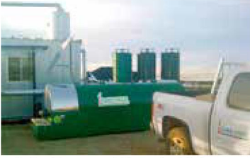
Solar Powered Chemical Injector
