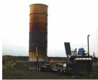
2 Million SCFD, Sweet Incinerators
