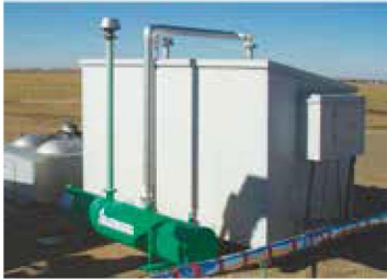
Scrubber Sweetening Systems
