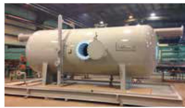
ESD Knockout Tanks
