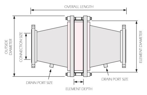
NOTE: 16" AND LARGER SIZES INCORPORATE CLASS 175 PRESSURE VESSEL FLANGES AT THE ELEMENT SECTION. ALL REMAINING FLANGES ARE 150 ANSI RATING.
