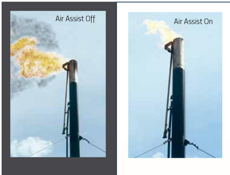
Smokeless Air Assist and Gas Assist complete with Silicon Nitride Retractable Pilot
